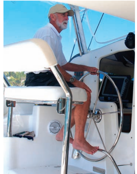
BELOW Owner Owen Day at the very ergonomic helm. The seat caters for two and collapses back, providing unimpeded standing room.
