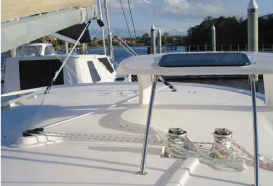
All sailing equipment can be operated from the cockpit; note the simple but effective 'traveller' system at the aft end of the hardtop.
