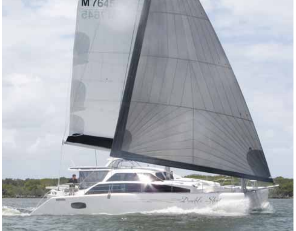
Powered up with screecher, it doubles the sailplan size. Alternatively the self-tacking jib is the standard option for easy sail handling.
